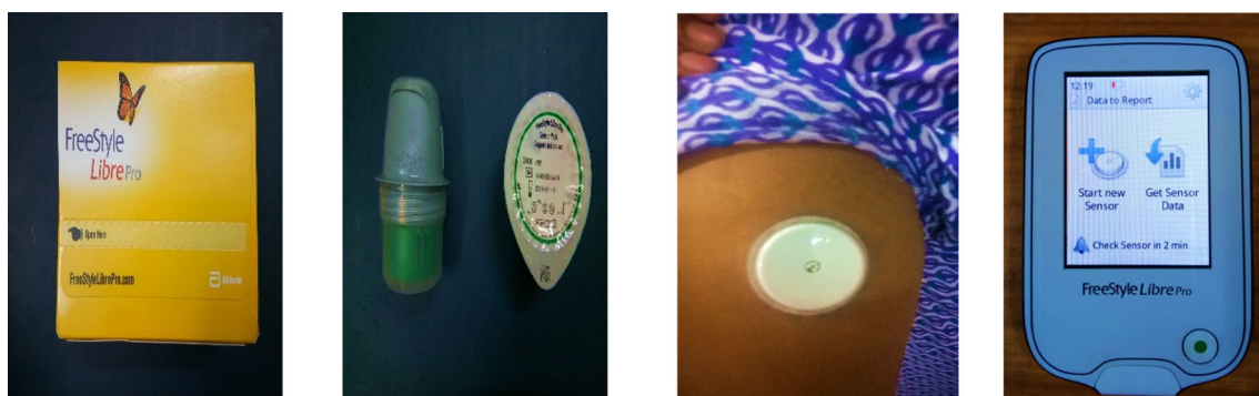
Fig. 1 FreeStyle Libre flash glucose monitoring system. a Flash glucose monitoring system. b Flash glucose monitoring applicator and sensor pack. c Flash glucose monitoring sensor. d Flash glucose monitoring reader
